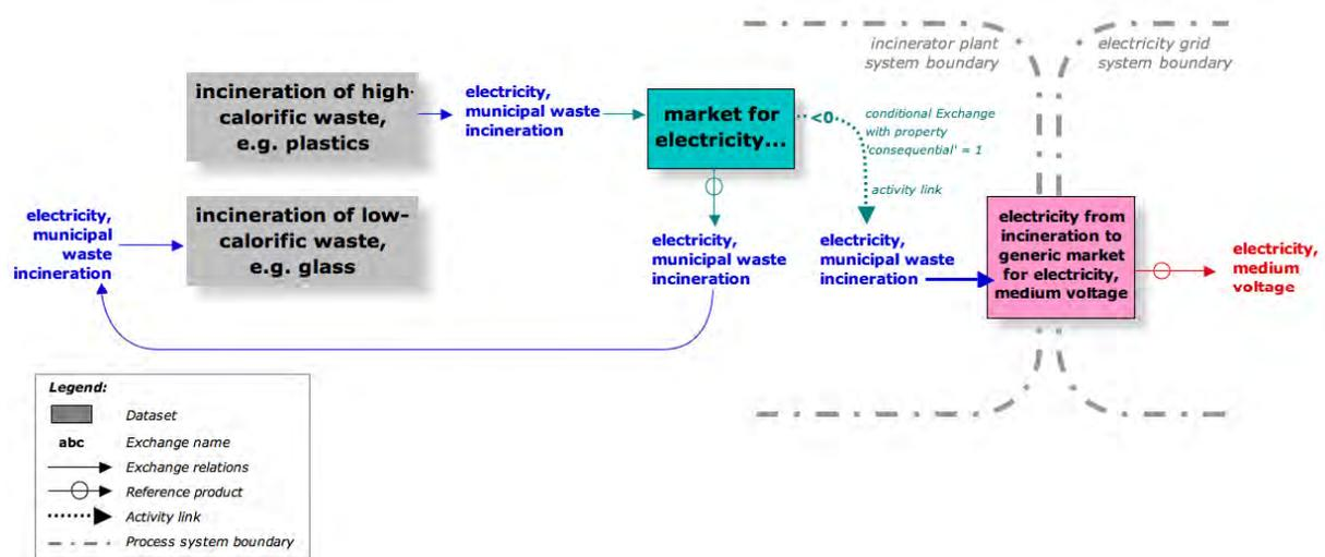
**Fig. 2.5** Extended scheme of internal electricity redistribution for a consequential System Model. The (constrained) market (blue-green box in centre) contains a conditional activity link to the "name changer" dataset for release to external grid market (right).
