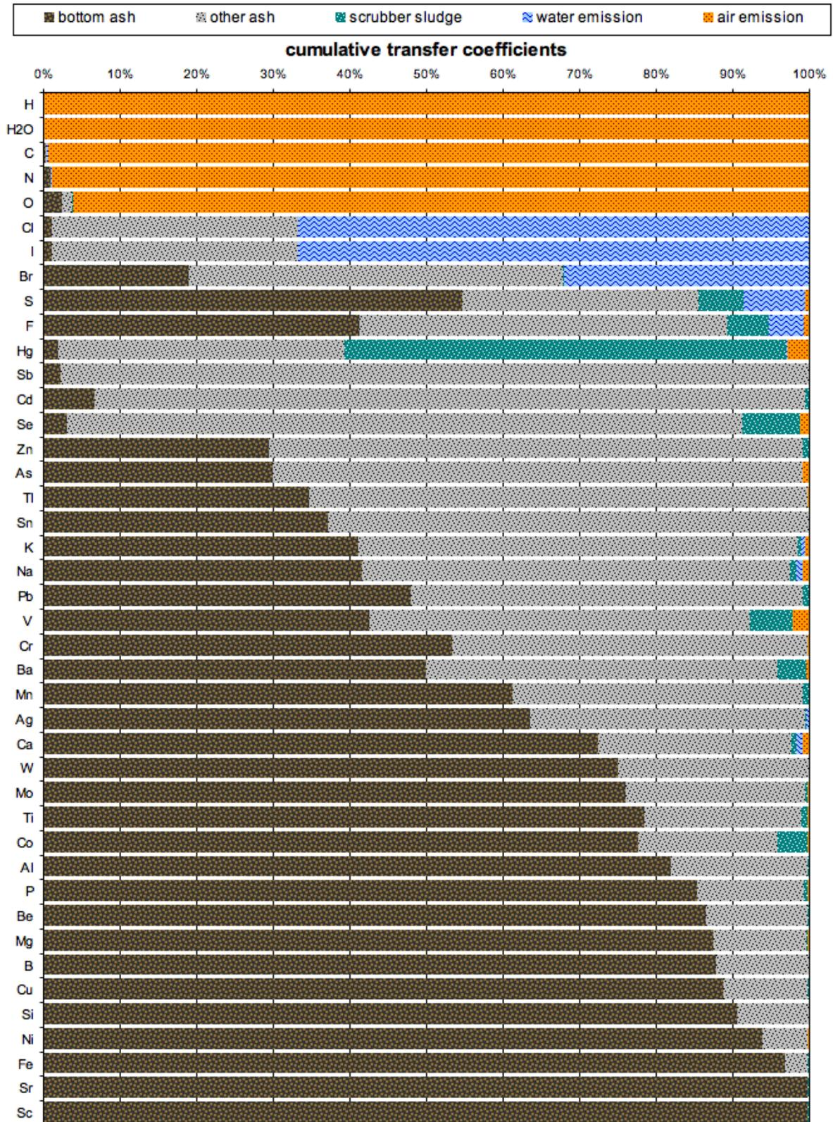
Fig. 6.1 Transfer coefficients for *burnable* waste in municipal waste incinerators
