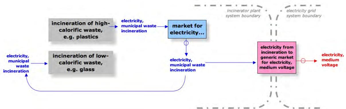
**Fig. 2.4** Scheme of internal electricity redistribution between incineration datasets for high- and low-calorific wastes (left) and the "name changer" dataset for release to external grid market (right). "electricity, municipal waste incineration" (blue exchange) is the exchange for the internal electricity product ; "electricity, medium voltage" (red exchange) is for the produced net energy product. Analogous redistribution for internal heat product.
