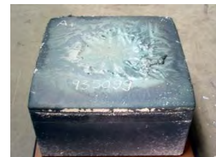
Fig. 5.9 400 kg ingot produced in Integrated Project Crystal-Clear. Source: Deutsche Solar, Germany
